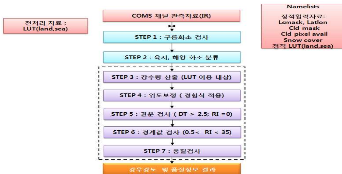
Figure 9. The Schematic diagram for the RI DPM procedure.
